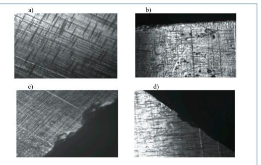
Fig. 27. Image of an injection section piston surface: a) a new piston surface fragment (the grinding traces clearly dominate), b, c, d) the piston surface area after operation (125x zoom) [16]
