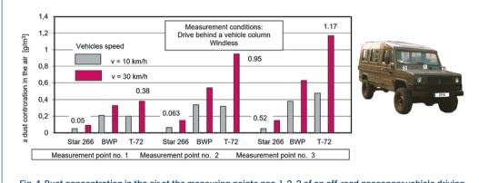
Fig. 4. Dust concentration in the air at the measuring points nos. 1, 2, 3 of an off-road passenger vehicle driving behind the column of: tanks T-72, BWP, Star 266 cars at different speeds [7]
