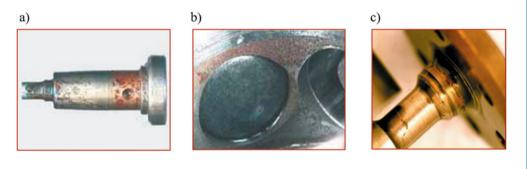
Fig. 35. Corrosive wear of the injection system components at inadequate water filtration: a) injector element corrosion, b) high pressure pump housing [10], c) valve in the Delphi injector [15]
