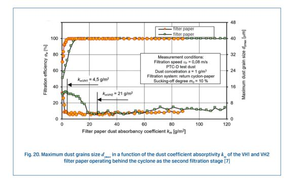
The dust grain smallest size ( $d_{zmax}$  = 2.7 µm) was recorded in the stream of the air purified by the VH1 filter paper at the absorbency coefficient  $k_m$  = 4.5 g/m<sup>2</sup>. However, in the air behind the VH2 paper, the maximum dust grain size  $d_{zmax}$  = 2.7 µm was recorded much later, only after the paper's reaching the absorbency coefficient  $k_m$  = 21 g/m<sup>2</sup> – Fig. 20.
