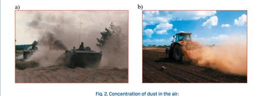
a) when a column of infantry's combat vehicles drives along the sandy ground (own source), b) during field works [17] During a sandstorm, the dust concentration in the air reaches  $10 \text{ g/m}^3$  [19]. Therefore, it is over 1,000 times greater than during the movement of vehicles on the streets.
