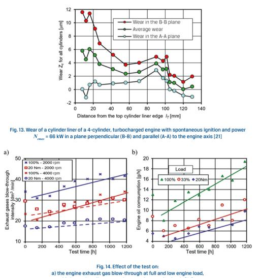
b) the engine oil consumption at various engine loads [21]
