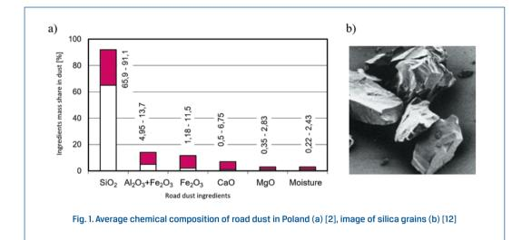
higher than the construction materials used in engines construction. The dust grains have usually very irregular shape (Fig. 1b), similar to polyhedral with sharp edges.
