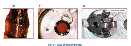
a) on the Delphi Nissan Micra 1.5 DCI's valve: b) in the Common Rail injector Delphi Ford Mondeo TDCI's valve seat [16], c) in the CPI high pressure pump suction valve [7]
