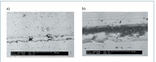
Fig. 11. Cracks in the cylinder bearing surface caused by dust particles [9]
